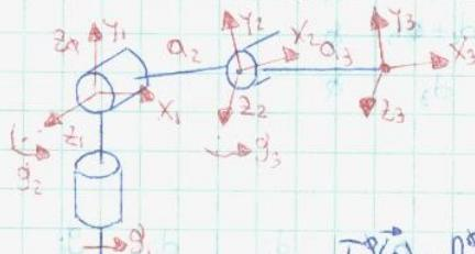
$$\text{NB: } \vec{J} = \begin{bmatrix} \frac{\partial P}{\partial g_1} & \frac{\partial P}{\partial g_2} & \frac{\partial P}{\partial g_3} \\ \vec{z}_0 & \vec{z}_1 & \vec{z}_2 \end{bmatrix}$$
