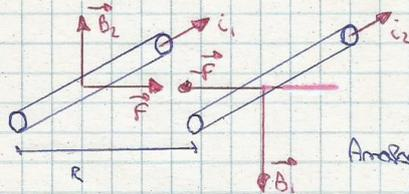
$$d\vec{F}_{1,2} = i_2 d\vec{s}_2 \times d\vec{B}_1 = \frac{\mu_0 i_1 i_2}{4\pi} \frac{d\vec{s}_2 \times (d\vec{s}_1 \times \vec{U}_1)}{R^2}$$
