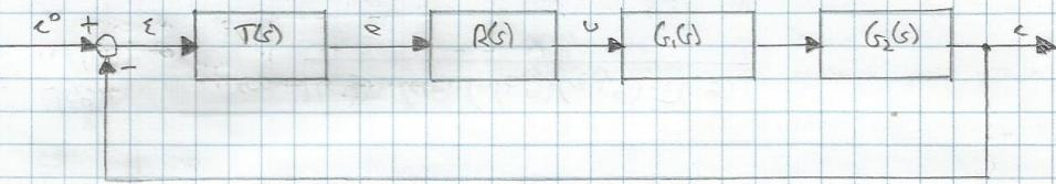
$$L(s) = T(s)R(s)G_1(s)G_2(s) \Rightarrow F(s) = \frac{L(s)}{1+L(s)}$$
